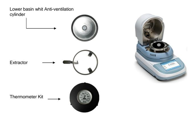
2. Position the lower basin whit anti-ventilation cylinder and calibration kit.
