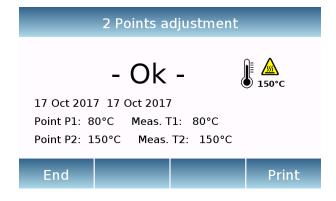
Press "End" to exit the adjustment function or "Print" to print the thermometer calibration data.
