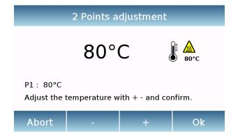
At the end of the first cycle, an acoustic signal will be output to open the oven cover and immediately read the temperature value on the thermometer.
