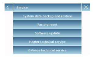
2. This will be accessed at the service menu. Select the function **Heater technical service**This feature is only accessible with a password: 1122, once typed correctly, press "OK".
