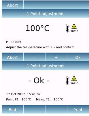
Correct the error using the "+" or "-" keys to correct the temperature. Once the correct temperature has been reached, press "OK" to confirm.
