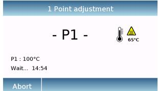
At the end of the cycle, an acoustic signal will be output to open the oven cover and immediately read the temperature value on the thermometer.
