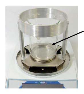
**2.** Place the **Beaker** in the correct seat of the support.
