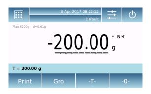
To reset the balance, remove all items from the plate and press the "- 0 -" key.
