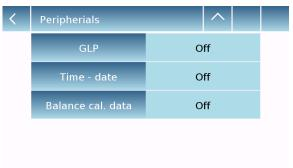
Tapping the parameter key to be set will activate its screen with the list of the various selectable options.
