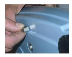
**Level** the balance by adjusting the legs on the front of the balance.
