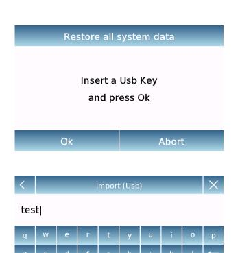
Insert the USB stick into the USB port on the left side of the device, and press the "OK" key.
