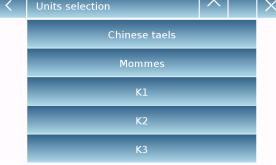
N.B.: The measurement unit selection can also be made directly from the weighing screen; by tapping the symbol of the current unit displayed, you will have access directly to the list of available units.
