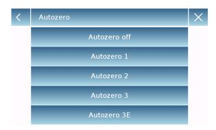
• Autozero: automatic zero correction constantly adjusts the zero value. These variations may be due, for example, to dirt that can be deposited on the plate. You can disable this function by selecting "Off" mode. Level 1 is the one with minor correction until it reaches level 3E which is the maximum correction.
