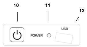
After connecting the power supply unit to the mains, the device will start automatically without having to press the power button.
