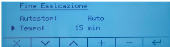
The default cycle time is 15min, so use the keys **+** **|** **-** to increase or decrease the value. Keeping the key pressed for a long time, the value is increased or decreased rapidly.
