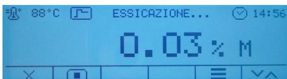
After closing the heater, the analysis cycle will be started.
