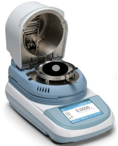
2. Position the lower basin whit anti-ventilation cylinder and calibration kit.
