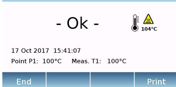
Press "**End**" to exit the adjustment function or "**Print**" to print the thermometer calibration data.
