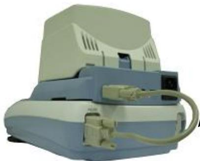
1. 15 poles M/F cable for connection balance-heater
