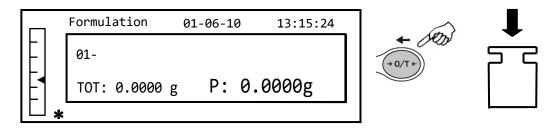
3. Carry out a tare operation if necessary, and load the first ingredient.
