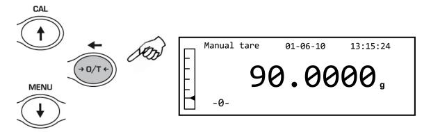
4. After having entered the desired value, press the **PRINT** button to confirm it. The value will remain in memory until the **TARE** button is pressed, or the instrument is disconnected from the power supply.
