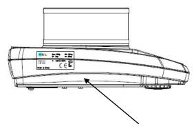
Position of the seal mark for Verified balances models
