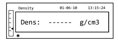
11. Now press the **ON/OFF** button to exit from the density function, or the **MENU** button to carry out the density measurement for another solid.
