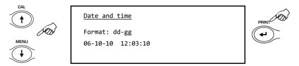
3. Set the desired date and time by using the **MENU** and **CAL** buttons to increase and decrease the number and the **PRINT** button to pass to the next date.
