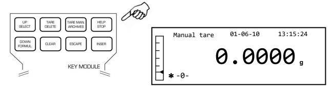
2. Press the **CLEAR** button to zero the preceding value and enter the new value, using the numerical keys on the lower part of the alphanumeric keypad.
