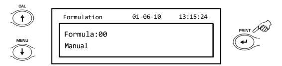
2. Select the number of the formula to save or modify using the **CAL** and **MENU** buttons to increase and decrease the value, after the word 'Formula'. Then press and keep pressed the **PRINT** button until the beeping stops to confirm the selection and enter the 'setup formula' menu.
