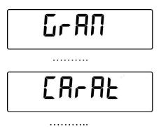
3. Press **PRINT** button to confirm or **MENU** button to shift to the other weight unit.
