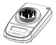
10. As soon as it is reached a sufficient number of pieces, this number is displayed and it will be possible to go on with count by loading the pieces count on the balance pan.
