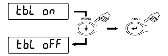
6. After you confirm with the **PRINT** button, the balance will restart automatically and will return to standard working mode.
