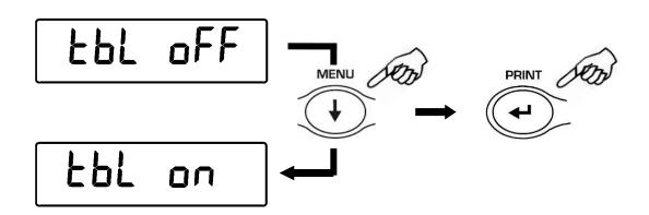
3. After you have choosen the mode "TBL ON" the balance will automatically restart and the message "TABLET" will appear on the display of balance. From this moment the interface device with the balance is the tablet.
