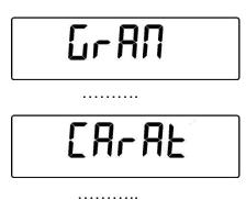
3. Press **PRINT** button to confirm or **MENU** button to shift to the other weight unit.
