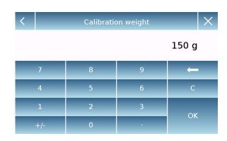
After selecting the "custom mode", tap the weight setting key to set the value of the desired weight.
