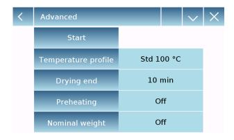
The display screen allows you to start a drying cycle tapping the "**Start**" key with the temperature parameters and modalities of the drying end displayed to the right of the function.
