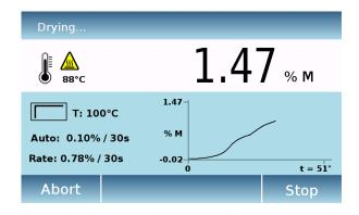
After closing the heater cover, the cycle will automatically start and the analysis screen will appear.
