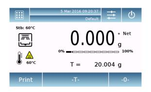
The **Net** symbol displayed shown the net weight. Tapping the "**Net**" symbol, you can display the gross weight "**Lrd**".
