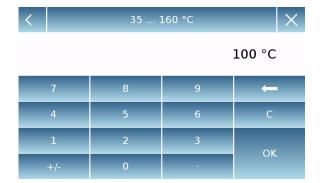
Standby temperature: this function allows you setting a maintaining temperature value for the heater.
