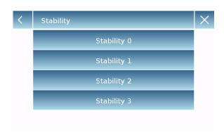
Stability: this function allows you to adapt the balance to environmental working conditions. When using the device in a low-vibration environment, select the Level 0. The default is Level 2. Use the Level 3 for very noisy environments.
