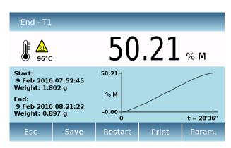
After recalling the last result, it will be displayed the same screen of the test end. In addition to display various drying parameters and the corresponding chart, you can perform the same test end operations:
