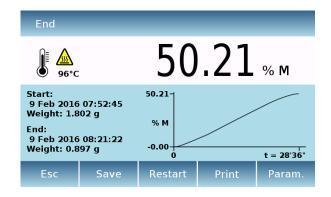
At the end of drying you will hear a short beep and display an "End" drying screen You can tap the unit of measure to change the display of the drying parameter or tap the graph to display it in full screen.
