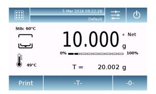
Place the material to be weighed on the balance and wait until the stability symbol turn on before detecting the value.
