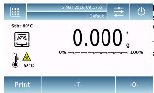
In simple weighing screen, the weight display area shows the value of the weight loaded on the weighing pan.
