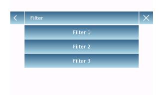
Filter: the filter function allows speeding up or slowing down the response of the balance depending on the weighing needs and environmental conditions. Selecting the level 1, the response will be immediate but the balance will be more sensitive to environmental disturbances such as ventilation and vibration. Increasing the level, the response will be slower and the indication will be more stable.
