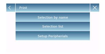
**Print:** the print function allows you to print on paper or on a drying program file by entering the name or by selecting it from a list.
