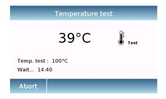
After starting the test, wait that the timer set automatically to 15 minutes is reset. You will hear a beep, so open the heater and compare the temperature value displayed with the one recorded by the thermometer placed inside
