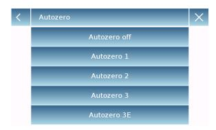
Autozero: automatic correction of zero constantly adjusts the value of zero. These possible changes may be, for example, due to dirt that may deposit on the pan. You can disable this function by selecting the "Off" mode. The Level 1 is the one with minor corrections until you get to Level 3E where the correction is maximum.
