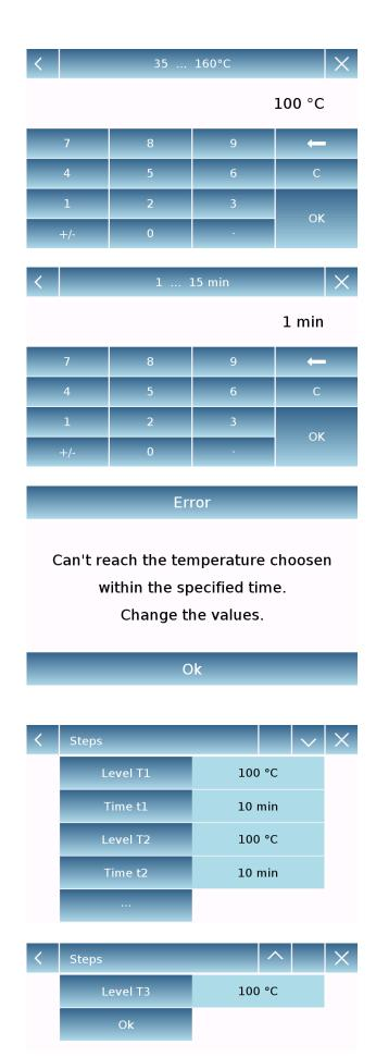
Tap the "**Temperature**" key to enable the alphanumeric keypad and enter the value desired. Then press "**Ok**".
