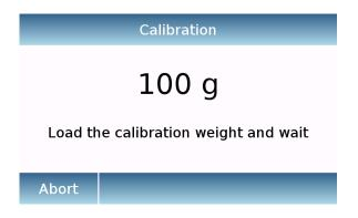
Load the required calibration weight or tap the "**Abort**" key to cancel the calibration procedure.
