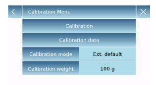
In the calibration menu you can perform the calibration, display and print data for the last calibration and set the calibration mode.
