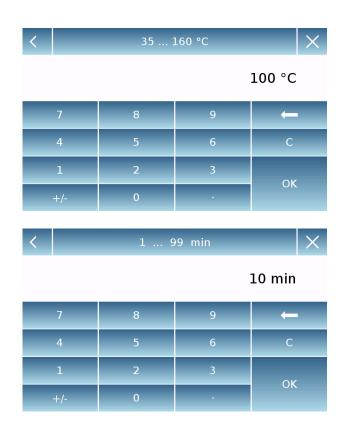
For the entry of the temperature and time, the numeric keypad will activate. Enter the value of the temperature and time, then press "**OK**" to confirm the value.
