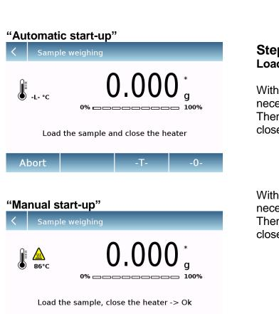
Abort Ok -T- -0- With "nominal weight" ON, load the quantity of substance set respecting the required tolerances.
