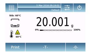
If you work with weighing containers, first zero the balance. Place the container and press the "-T-" key.
