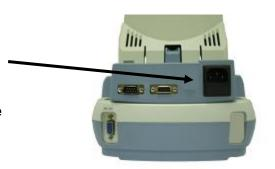
So **connect** the VDE cable to the outlet in the vicinity of the device. Do not use cables/extensions non-compliant with current regulations.
