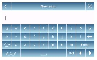
It will then automatically activate the keyboard for entering the user name. The maximum allowed number of characters is equal to 30.
