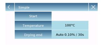
The display screen allows you to start a drying cycle by tapping the "**Start**" button with the temperature parameters and modalities of the drying end displayed to the right of the function.
