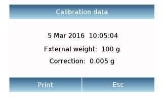
Calibration data: in the calibration data screen, you can check the date of the last calibration, the manner in which it was performed, the value of the weight used and the correction made since the previous calibration. Tapping "Print", you can print out the displayed data.
