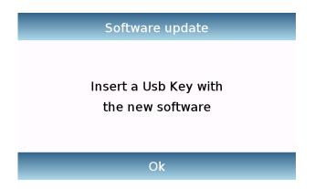
Insert the USB stick in the port on the left side of the device by checking before the update program provided by the manufacturer is loaded on the stick and confirm with the "**OK**" button.
