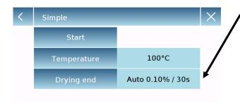
**Time:** setting this method of the end drying, the cycle will end when the time set will be elapsed. Also you can end the cycle manually at any time by tapping the "**Stop**" key. Enter the value of time and press the "**OK**" button to confirm
