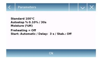
**Param.:** tapping the "Param." Key, you can display all parameters used for the drying cycle.
