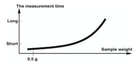
Therefore, based on the substance, it's necessary to determine the right compromise between the drying time and the accuracy of the results you want to obtain.
