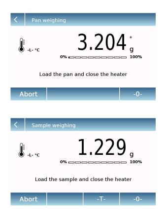
**Load the substance** to analyze and close the oven.
