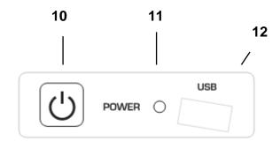
After inserting the power cord, the device will start automatically without having to press the power key.
