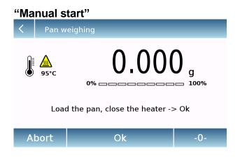
With the "Manual" start mode, reset if necessary by tapping " – 0 – "
