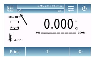
After unlocking the user in the basic screen on the left side of the user name, you will display an open padlock.
