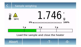
After reached the minimum value, the bar changes color and turns green, indicating that the quantity loaded is within the set limits. It will then remain in this color range until it is
