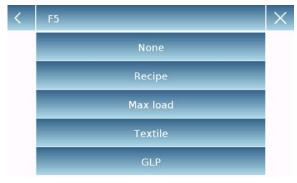
To remove a function, press the key corresponding to the function you want to remove and select "**None**" in the list.
