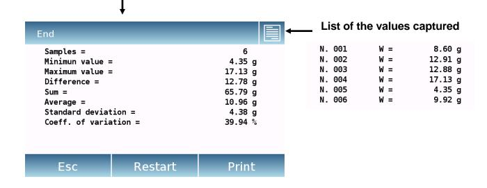
Tap the "Esc" key to exit the function, the "Restart" key to make a new measurement and the "Print" key to print the measurement result.
