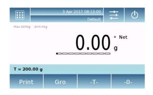
The **Net** symbol on the display indicates the net weight. Press "**Net**" to see the gross weight "**Lrd**".
