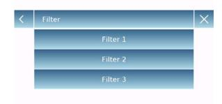
Filter: the filter function allows to speed or slow down the balance response according to weighing requirements and environmental conditions. By selecting Level1, the response will be immediate, but the balance will remain more sensitive to environmental disturbances such as ventilation and vibration. By increasing the level, the response will be slower and the indication more stable.
