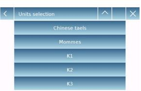
On the "**Units Selection**" screen, all available weighing units are immediately displayed. Tap the desired unit to select it and enable it.
