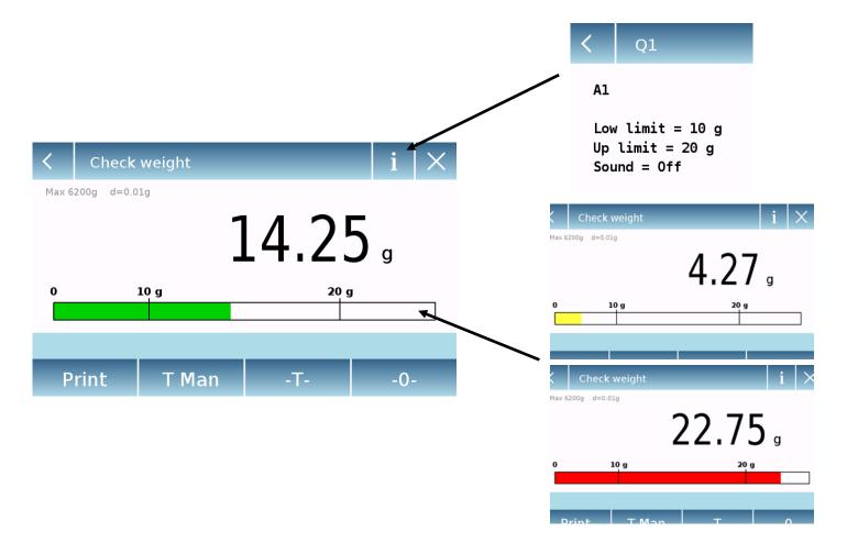
The Check weight bar is yellow when the loaded weight is lower than the minimum threshold and green when the weight is within the set range (with the beep indication when activated) and red when the weight is greater than the upper threshold set.
