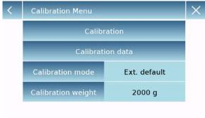
In the calibration menu, you can calibrate, display and print the data for the last calibration and set the calibration mode.
