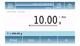
Place the material to weight on the balance and wait for the stability symbol to light up before detecting the value.
