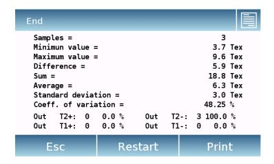
Tap the "Esc" key to exit the function, the "Restart" key to make a new measurement and the "Print" key to print the measurement result.
