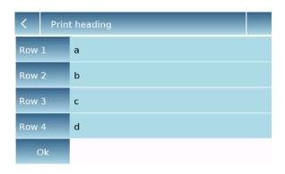
In the print header screen, tap the rectangles that indicate the line number to automatically enable the alphanumeric keypad and enter the desired text with a maximum number of 40 characters per line.
