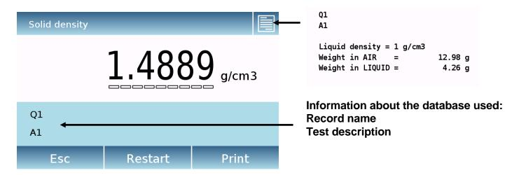
Tap the "Esc" key to exit the function, the "Restart" key to make a new measurement, and the "Print" key to print the measurement result.
