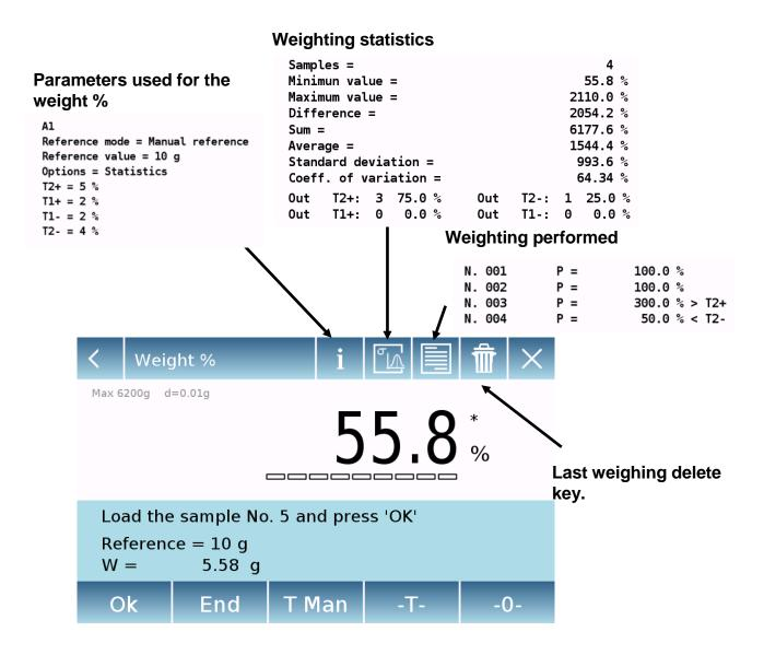
Tap the "Ok" key to capture a new weight and tap the "END" key to end the capture and perform the final statistical calculation.
