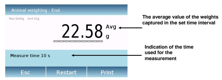
Tap the "Esc" key to exit the function, the "Restart" key to make a new measurement and the "Print" key to print the measurement result.
