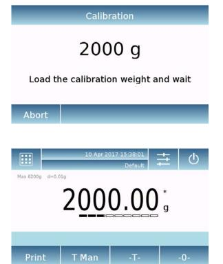
Load the required calibration weight or tap the "**Abort**" button to cancel the calibration procedure.
