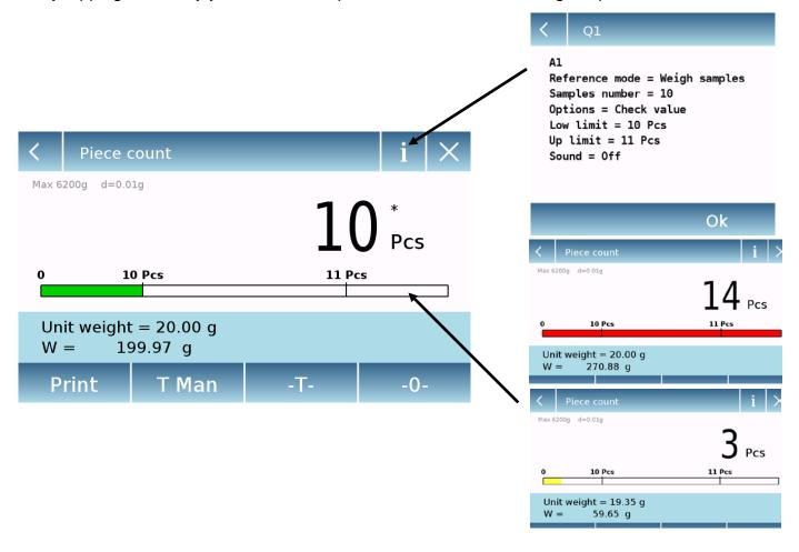
The pieces number control bar is yellow when the number of pieces loaded is lower than the minimum threshold. It is green when the pieces are within the set range (with the beep indication when activated) and red when the number of pieces exceeds the upper threshold set.
