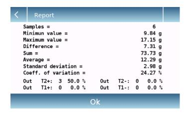
After tapping the "End" key, the screen with the result of the weighing statistics is displayed.
