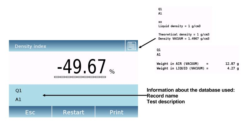
Tap the "Esc" key to exit the function, the "Restart" key to make a new measurement, and the "Print" key to print the measurement result.
