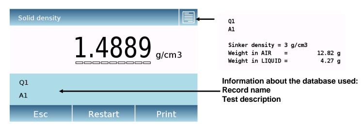
Tap the "**Esc**" key to exit the function, the "**Restart**" key to make a new measurement, and the "**Print**" key to print the measurement result.
