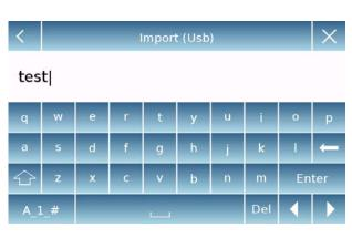
If the USB stick is inserted correctly, after confirmation, the alphanumeric keypad will automatically be displayed for entering the name of the backup you want to restore.
