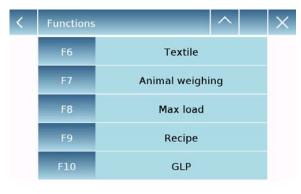
To assign a function, press the key you want to assign and select one from the list of available functions.
