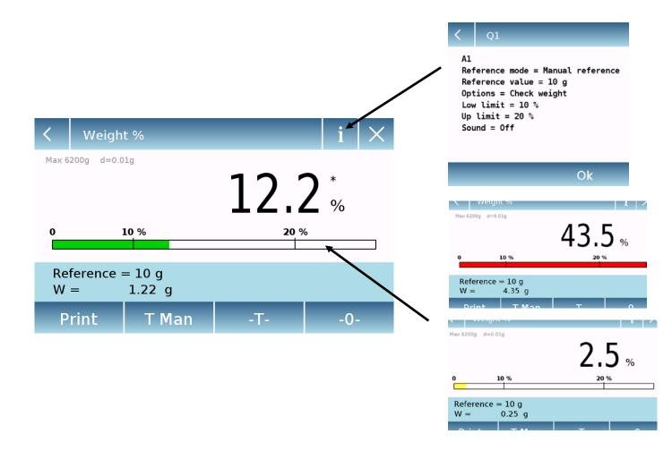
The weight check bar is yellow when the loaded weight is lower than the minimum threshold, green when the weight is within the set range (with the beep indication when activated) and red when the weight is greater than the upper threshold set.
