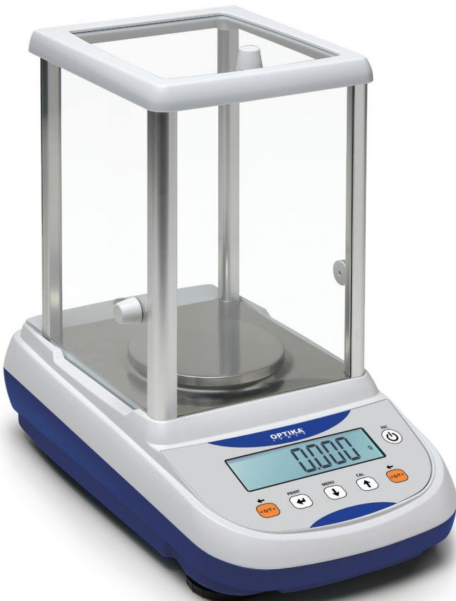
CH models are equipped with a large glass draught shield.
