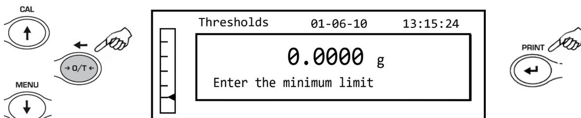
2. Enter the MINIMUM limit value by using the **CAL** and **MENU** buttons to increase and decrease the value, while pressing the **O/T** button to pass to the next number. During the entering phase, prolonged pressure on the **O/T** button allows you to delete the entered value.
