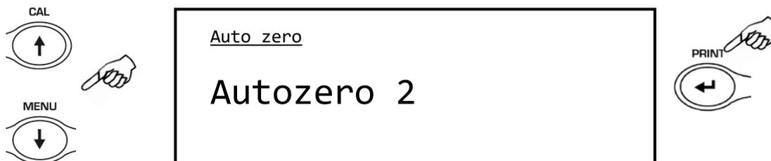
2. Select the desired autozero level. By pressing the **MENU** or **CAL** button it will be possible to scroll through the various levels forward or backward; then confirm your choice with the **PRINT** button.
