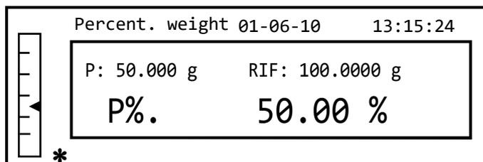
5. Now remove the reference weight, load the sample and read the percentage weight.
