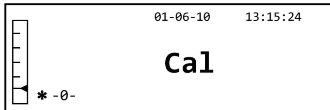
2. At the end of the calibration, the balance will return to normal weighing conditions.
