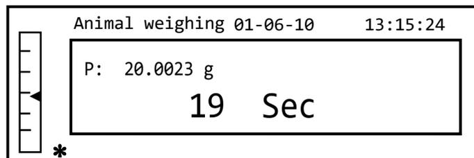
4. Once acquired, the weight will be shown on the display with an indication of the average weight detected.
