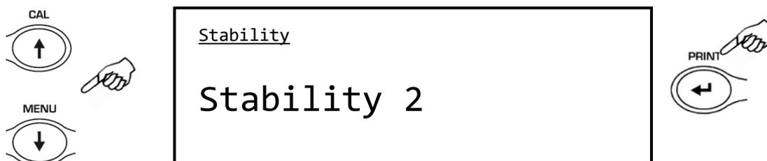
2. Select the desired stability level. By pressing the **MENU** or **CAL** button you can scroll through the various levels forward or backward; then confirm your choice with the **PRINT** button.
