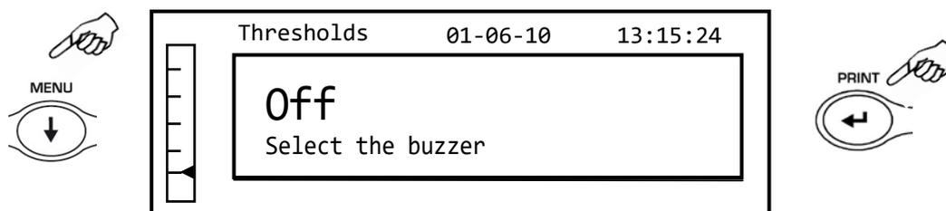
8. Through the **MENU** key, select the activation or not of the acoustic signal when the weight is within the two set limits. Then confirm the selection by pressing the **ENTER** button.
