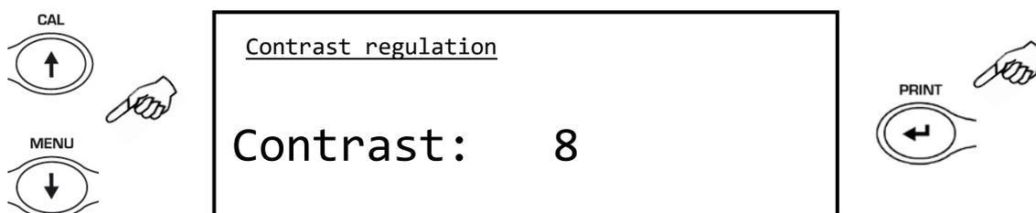
3. After having selected the desired contrast level, the screen relative to the balance parameters menu will be displayed again. It will now be possible to select another parameter or return to weighing mode by pressing the **ON/OFF** button.
