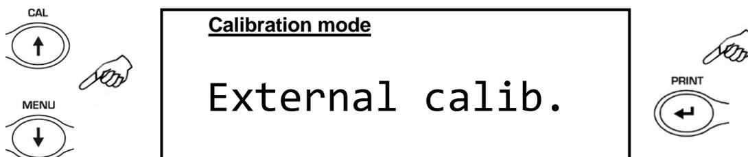
2. Select the desired mode. By pressing the **MENU** or **CAL** buttons it will be possible to scroll the different calibration modes forward or backward:
