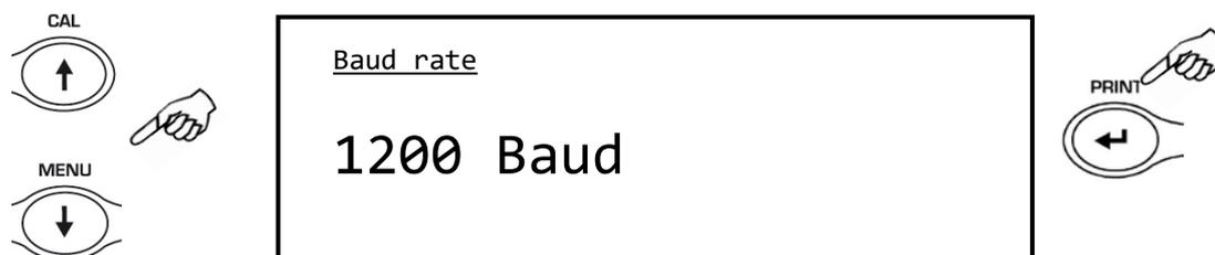
2. Select the serial data transmission speed (1200-2400-4800-9600 baud). By pressing the **MENU** or **CAL** button you can scroll the different transmission speeds forward or backward; then confirm the choice with the **PRINT** button.
