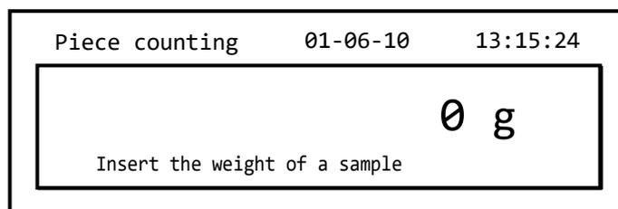
1. Insert the unit weight in grams of the sample by using the numeric keys from 0 to 9 and the decimal point.
