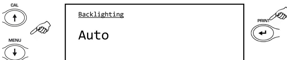
2. Select the desired modality. By pressing the **MENU** or **CAL** button it will be possible to scroll through the various levels forward or backward; then confirm the choice with the **PRINT** button.
