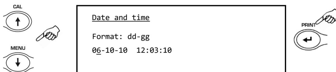
4. After having regulated the date and time, press and hold the **PRINT** button until the beeping stops and then release the button to save the settings.
