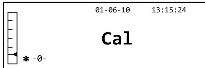
2. When the value of the calibration weight begins to flash, load the weight indicated by the display on the plate.
