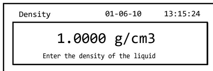
4. It is possible to insert a different value using the **CAL** and **MENU** buttons to increase and decrease the value, while pressing the **O/T** button to pass to the next value. During the entering phase, prolonged pressure on the **O/T** button allows you to cancel the inserted value.
