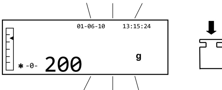
3. The display will stop flashing, indicating the value of the calibration weight with the stability indicator on.
