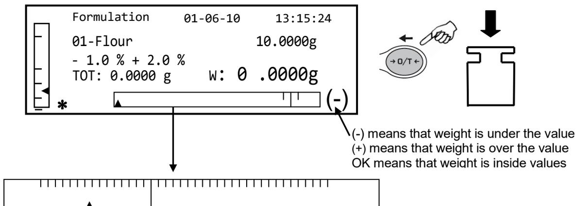
To facilitate the dosing operation, when the value of the component is approaching the threshold of the acceptable value, the dosing bar will automatically zoom.
