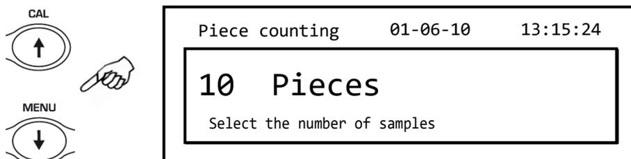
1. Select the number of pieces to put on the plate as a sample, pressing in sequence the **MENU** button to increase and the **CAL** button to decrease.
