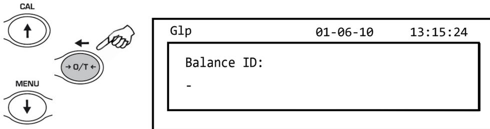
2. Enter the balance ID (it can be a series of numbers or letters, max 18 characters) using the **MENU** and **CAL** buttons to scroll through all of the available characters. To select uppercase or lowercase characters, press and hold the **MENU** button until the beeping stops.
