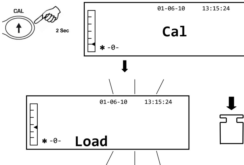
2. Load a weight that is equal to or greater than the pre-set calibration weight on the plate; the balance will recognize a weight that is equal to or greater than the calibration weight as valid provided that it is a whole weight with respect to the most significant figure of the calibration weight.
