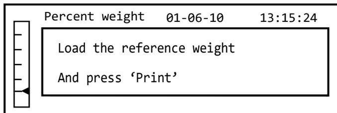
4. Load the reference weight on the plate and then press the **PRINT** button; the word "Wait" will be shown. Once the weight is acquired, a screen with an indication of the weight loaded, reference weight, and percentage weight will be shown.
