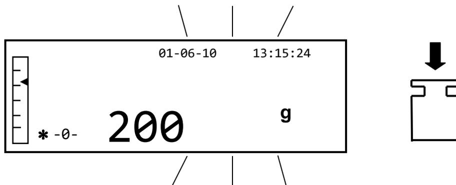
3. Wait for the calibrated weight to be displayed and the stability symbol to turn on, and then remove the weight from the plate.
