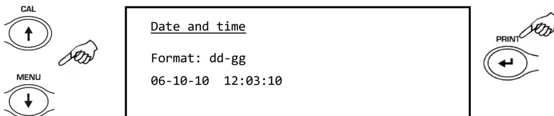
3. Set the desired date and time by using the **MENU** and **CAL** buttons to increase and decrease the number and the **PRINT** button to pass to the next date.
