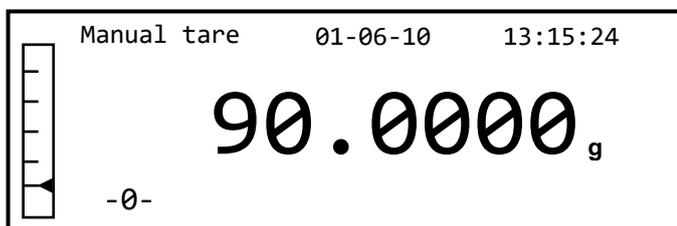
4. After having entered the desired value, press the **PRINT** button to confirm it. The value will remain in memory until the **TARE** button is pressed, or the instrument is disconnected from the power supply.
