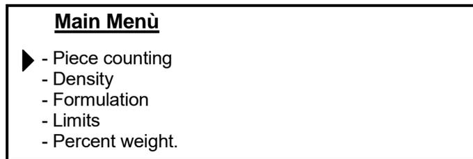
3. Now use the CAL and MENU buttons to navigate forward or backward in the menu of parameters.
