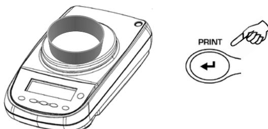
3. Load the number of pieces indicated on the display on the plate and press the **PRINT** button.
