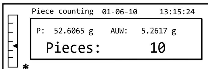
If the pieces to be counted have a weight that is too little with respect to the balance's resolution, an error message will be displayed.
