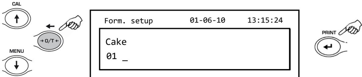
5. Enter the name of the first component (it can be a series of numbers or letters, max 11 characters) using the **MENU** or **CAL** buttons to scroll through the available characters.
