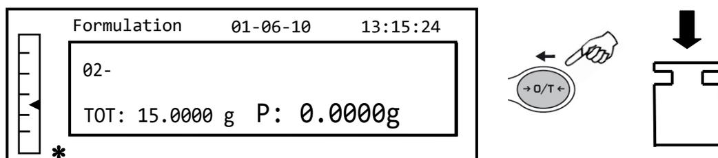
5. Carry out a tare operation if necessary, and load the second ingredient.
