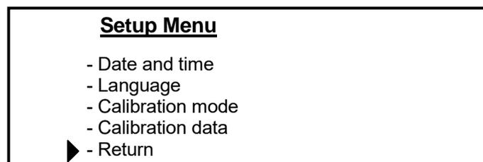
4. Position the cursor on the desired parameter and press the PRINT button to confirm the selection.
