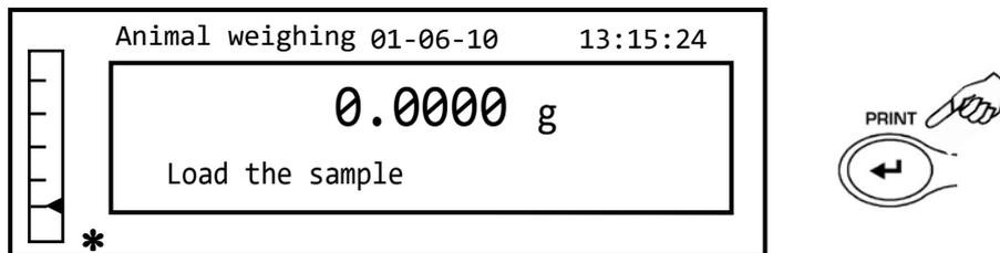
3. Load the sample to be weighed on the plate and press the **PRINT** button; the value of the current weight and the set sampling countdown time will be displayed.
