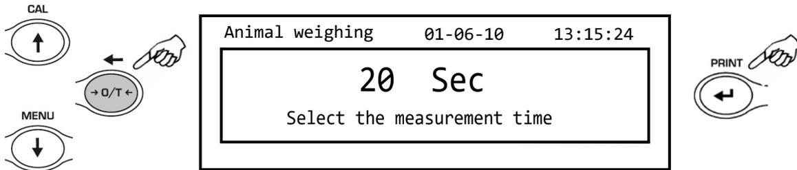
2. Set the desired time from 5 to 90 seconds using the **MENU** key to decrease and **CAL** to increase. Then confirm by pressing the **PRINT** button.
