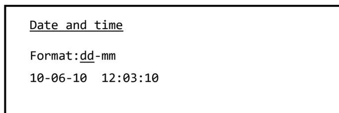
2. Select the desired format of the date. Pressing the **MENU** or **CAL** button it will be possible to modify the format dd-mm or mm-dd; then confirm the choice with the **PRINT** button.
