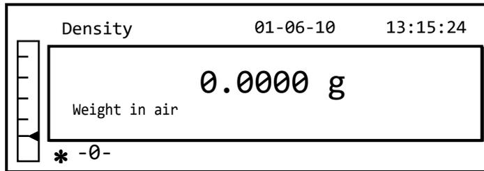
7. Carry out a tare if necessary and load the solid. Wait for the stability symbol to appear and press the **PRINT** button to acquire the value. The word 'wait...' will appear during the acquisition of the value.
