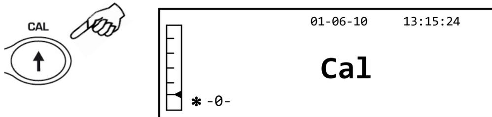
2. When the value of the calibration weight begins to flash, load the calibration weight on the plate.
