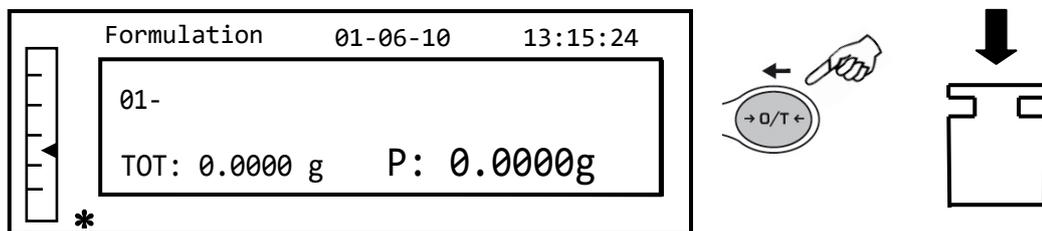
3. Carry out a tare operation if necessary, and load the first ingredient.
