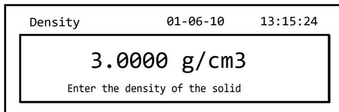
4. A different value can be entered by using the **CAL** and **MENU** buttons to increase and decrease the value, while pressing the **O/T** button to pass to the next value. During the entering phase, prolonged pressure on the **O/T** button allows you to delete the inserted value.
