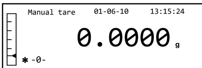
3. Now insert the desired tare value using the **CAL** and **MENU** buttons to increase and decrease the number, while pressing the **O/T** button to pass to the next number. During the entering phase, holding down the **O/T** button allows you to delete the inserted value.
