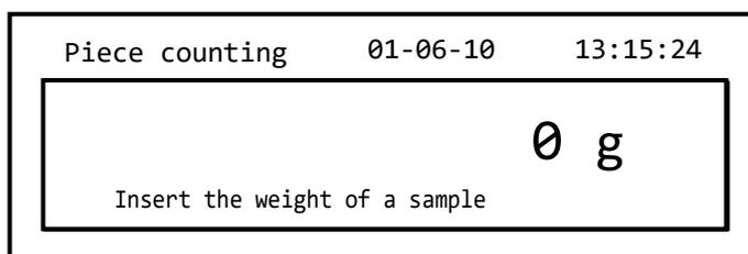
4. Insert the piece's unit weight in grams using the **CAL** and **MENU** buttons to increase and decrease the value, while pressing the **O/T** button to pass to the next value. To insert a decimal point, hold down the **CAL** button for a prolonged time. During the entering phase, the prolonged pressing of the **O/T** button allows you to delete the inserted value.
