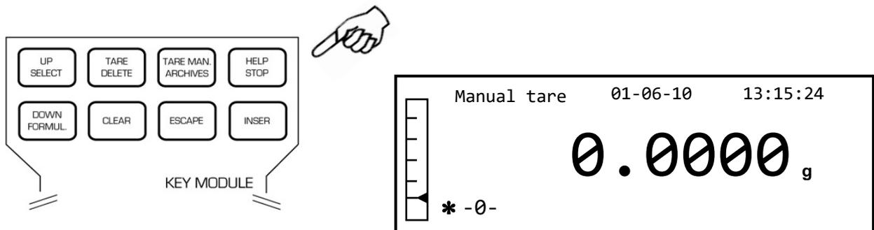
2. Press the **CLEAR** button to zero the preceding value and enter the new value, using the numerical keys on the lower part of the alphanumeric keypad.
