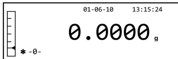
4. Put the objects to be weighed in the container. Read the value of the net weight on the display.
