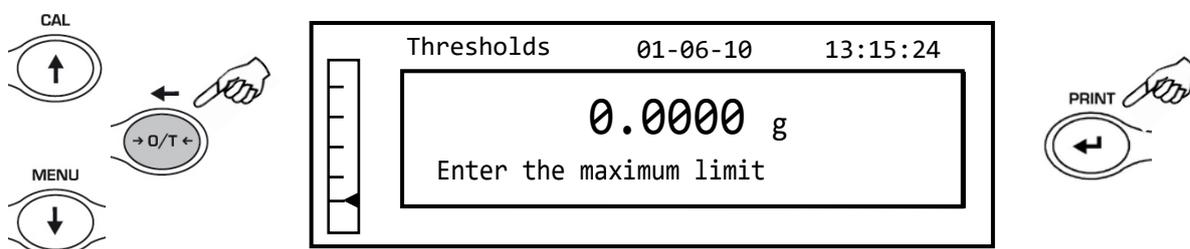
5. Now insert the MAXIMUM limit using the same procedure described for the insertion of the MINIMUM limit.
