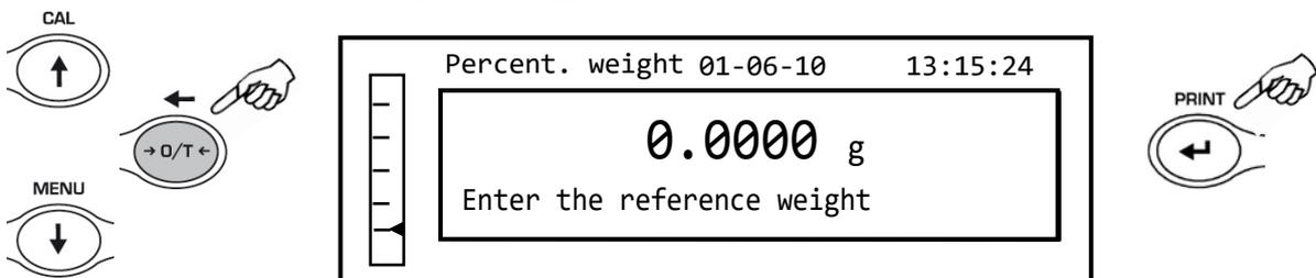
4. You can now enter the reference weight value, using the **CAL** and **MENU** keys to increase and decrease the value, while pressing the **O/T** button to pass to the next value. During the entry phase, holding down the **O/T** button allows you to delete the value entered. The value entered will remain in the memory until the balance is turned off. It is also possible to enter the value using the optional alphanumeric keypad.
