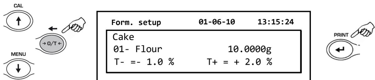
7. Now enter the quantity of the component using the **MENU** or **CAL** buttons to increase or decrease the value while pressing the **O/T** button to pass to the next value and the **PRINT** button to pass to the next parameter
