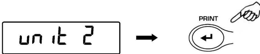
6. The "**GRAM**" unit will be displayed. Pressing the **MENU** or **CAL** key will now be possible to scroll backwards or forwards the secondary units menu.
