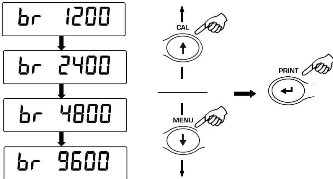
3. After having selected the transmission speed you wish, press the **MENU** button to go to next parameter or **CAL** button to go to previous one.
