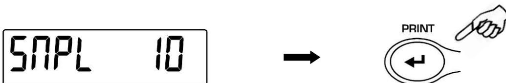
3. Load on the pan the number of pieces displayed on the balance display
