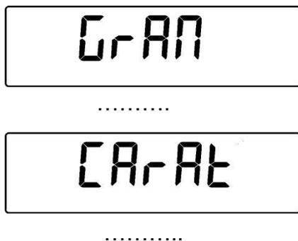
7. Press the **PRINT** key to confirm or **MENU** to change to another unit of measurement (the units of measurement available are the same as those listed in point 3).
