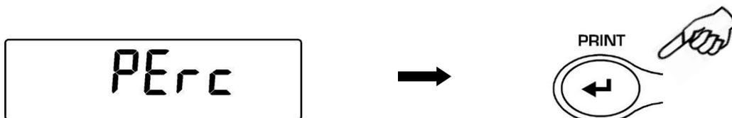
2. Press the **MENU** button to select the **“Perc A”** function and press **PRINT** button to confirm.
