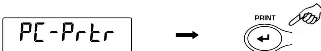
2. To select the data print mode, press **MENU** until the message “**PRINT**” is displayed or “**TLP50**” if you want to connect the TLP50 printer for printing on labels or on paper with date and time.
