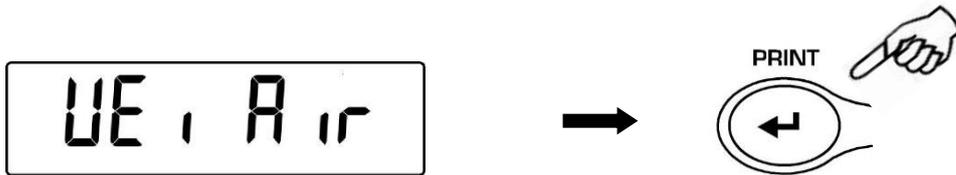
8. Now perform a tare if necessary and put the glass float to the weighing hook. Press then the **PRINT** button to acquire the value. During the acquisition of the value the message **WEI AIR** will be flashing.
