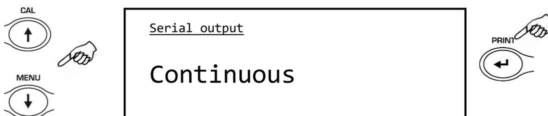
2. Now by pressing the **MENU** or **CAL** button it will be possible to scroll through the serial output **MENU** forward or backward.
