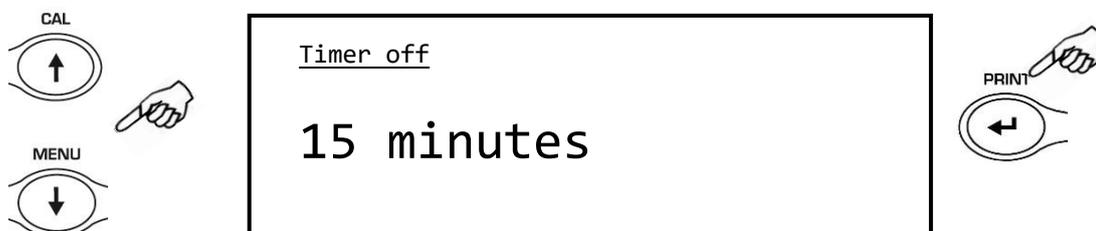
2. Select the desired auto-off modality. By pressing the **MENU** or **CAL** button it will be possible to scroll the various levels forward or backward; then confirm the choice with the **PRINT** button.
