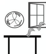
**Avoid** exposure to extreme temperatures and temperature fluctuations that occur, for example, if the device is placed closed to a radiator or in places under direct sunlight.
