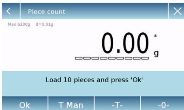
Carry out the container tare if necessary, in the case of sample counting before counting, it will be required to load the number of pieces chosen (for sampling) on the plate, while in the mode with average unit weight, you can go directly to the count of the pieces.
