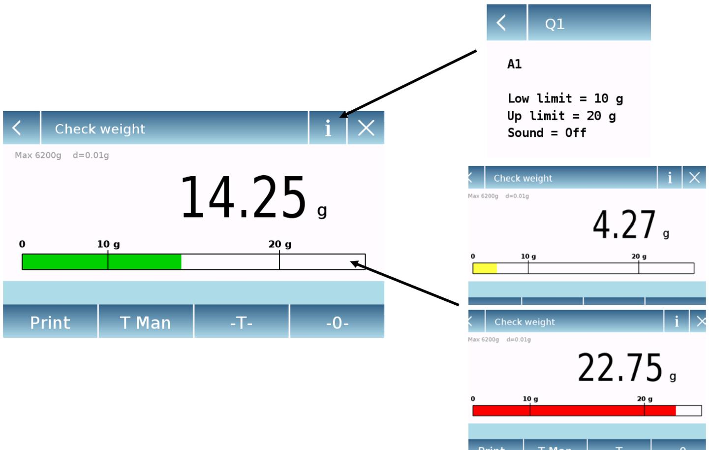
The Check weight bar is yellow when the loaded weight is lower than the minimum threshold and green when the weight is within the set range (with the beep indication when activated) and red when the weight is greater than the upper threshold set.
