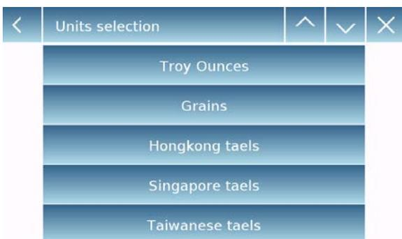
On the "**Units Selection**" screen, all available weighing units are immediately displayed. Tap the desired unit to select it and enable it.
