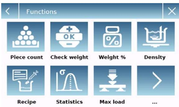
From the base weighing screen, tap
