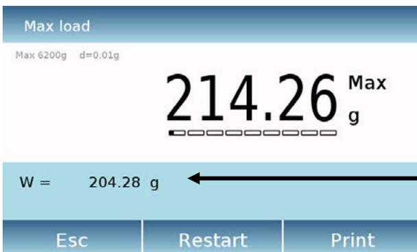
Once the tested sample breakage load is reached, the maximum weight will be displayed.
