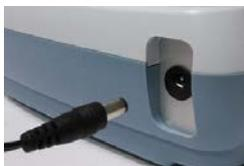
Plug the jack provided in the connector on the back of the instrument.
