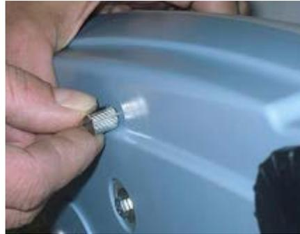
Level the balance using the level bubble and levelling feet located underneath the case.
